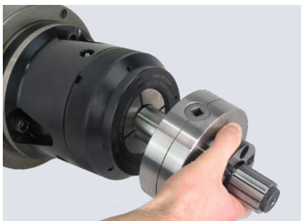
Load the KEM-MA manual actuator into a three jaw or collet chuck, gripping on the 38mm location spigot.
